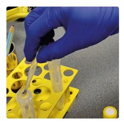
Collected samples can be processed in multiple ways, including direct fixation or further *ex-vivo* cultivations. The forceps are inert (fully compatible with organic fixatives), sterile, toxin- and pyrogen-free.
