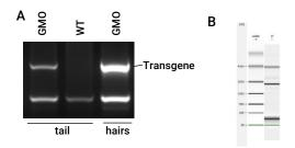
Collected hair samples can be used as a source of DNA and RNA. A) Results of genotyping of a transgenic mouse. The classical invasive approach of obtaining mouse DNA (tail clipping) is compared to the collected hairs' DNA. B) Assessment of mRNA quality isolated from hair follicular cells by miRNeasy mini kit (Qiagene) measured on Agilent RNA Pico Chip
